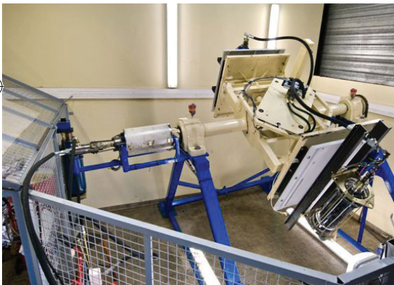
Accumulator test bench for wind turbine application.
